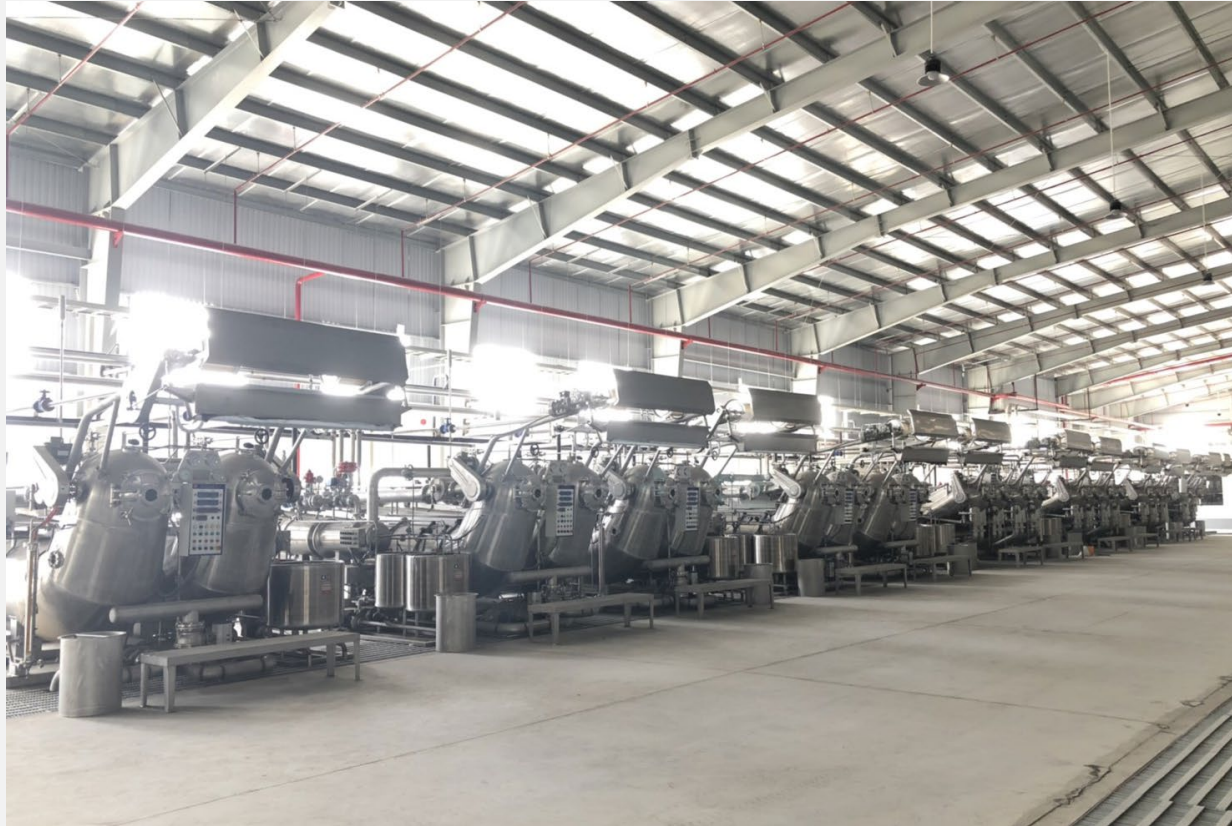
Extreme-rapid, High-temperature & High-pressure Jet Dyer
