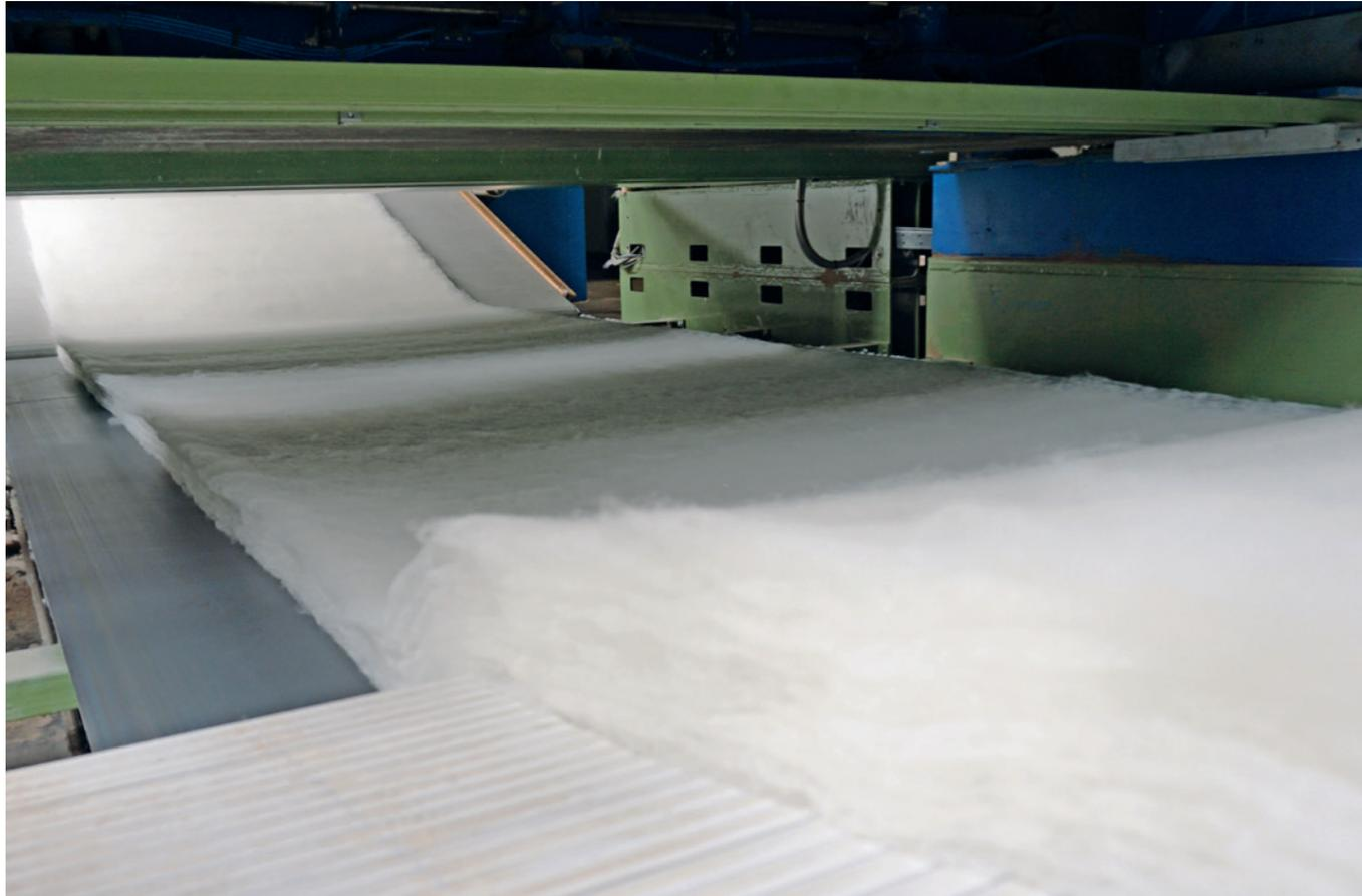
lavalan® insulation before the thermal bonding process
