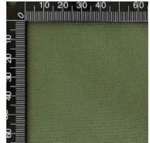
Design No: N0997 Content: 100% Re-Nylon Description: N400D*N400D Finishing: PD+C0 WR+PU600mm Remark: NE-15
