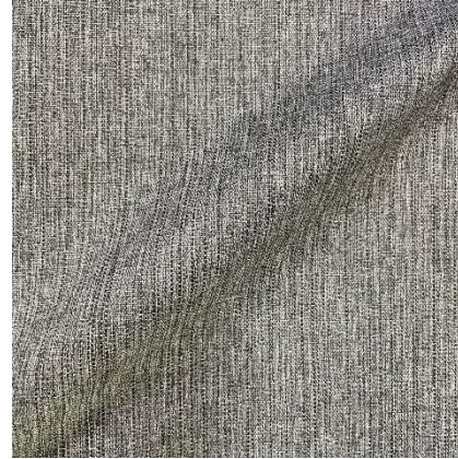
Design No: P1646-1 Content: 100% POLYESTER Description: T300D * T300D Finishing: CO WR+PU1500MM
