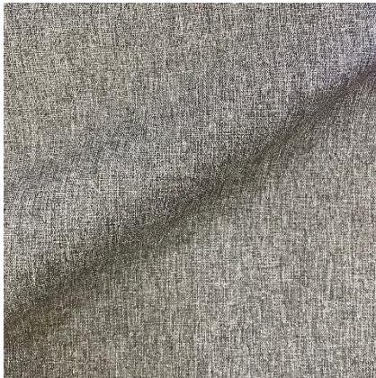
Design No: P1654 Content: 100% POLYESTER Description: T300D * T300D Finishing: CO WR+PU1500MM
