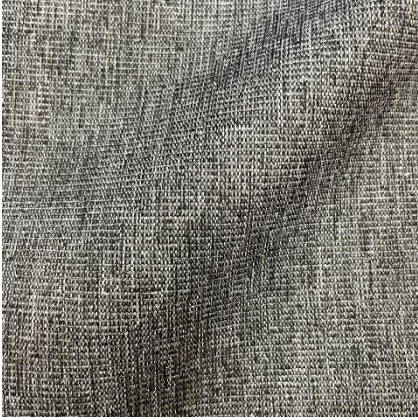
Design No: P1655-1 Content: 100% POLYESTER Description: T300D * T300D Finishing: CO WR+PU1500MM
