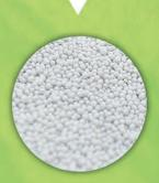
Bottle flake melted and formed into chip.
